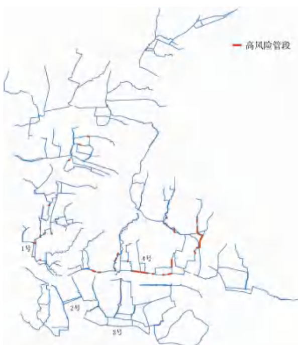
图7 建设连通管后的“高风险”管段分布 Fig. 7 Distribution of High Risk Pipe Sections after Construction of Connecting Pipes
