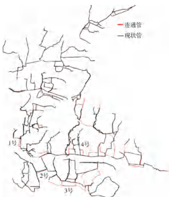
图6 中心城区污水干管现状管和连通管分布 Fig. 6 Distribution of Sewage Mains and Connecting Pipe in the Central Urban Area
